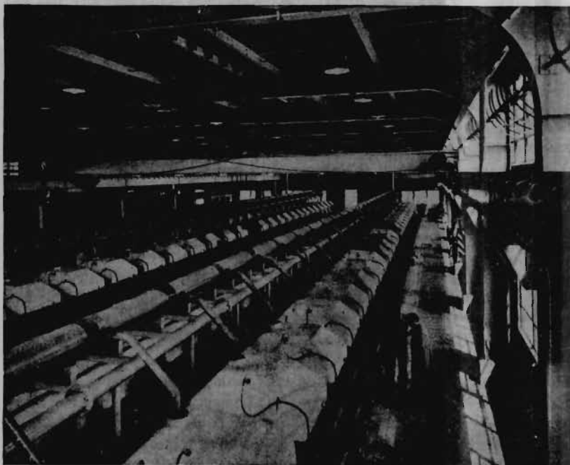
FIG. 8. Typical Hooker S-3A cell installation. (Courtesy of Hooker Electrochemical Co.)
