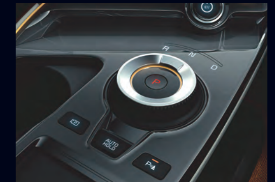
Shift By Wire Change gear position simply by turning the dial of Shift by Wire system left or right
