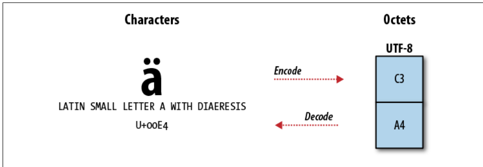
Figure C-1. The code point of a character is not its storage. The encoding transforms characters into storage.
