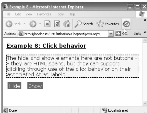
Figure 5-16. Two HTML <span> elements that have click behaviors associated with their Atlas controls
