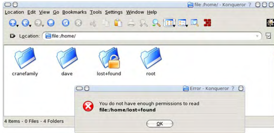
Figure 6.1 Various conventions for providing status information in a user interface: modifying the icons to reflect particular characteristics (here access permissions), a status bar providing summary information, and a modal dialog. The interface shown here is the KDE desktop for UNIX workstations, but similar conventions are found in most popular graphical interfaces.
