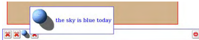
Figure 6.3 Messages on the status bar can be inspected by rolling the mouse over the icon, causing a tooltip to appear.
