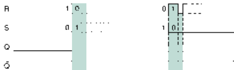
b. Timing diagram for circuit of Figure 6.13b
