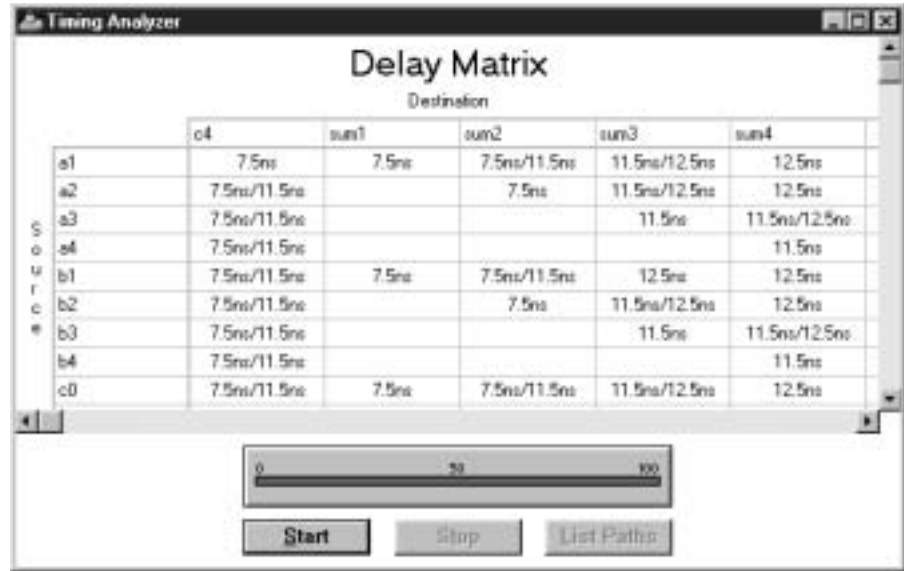
FIGURE 6.30 Delay matrix for a 4-bit adder (Normal Synthesis)
