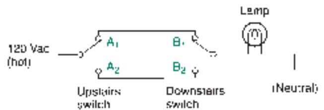
FIGURE 2.40 Problem 2.21: Circuit for Two-Way Switch
