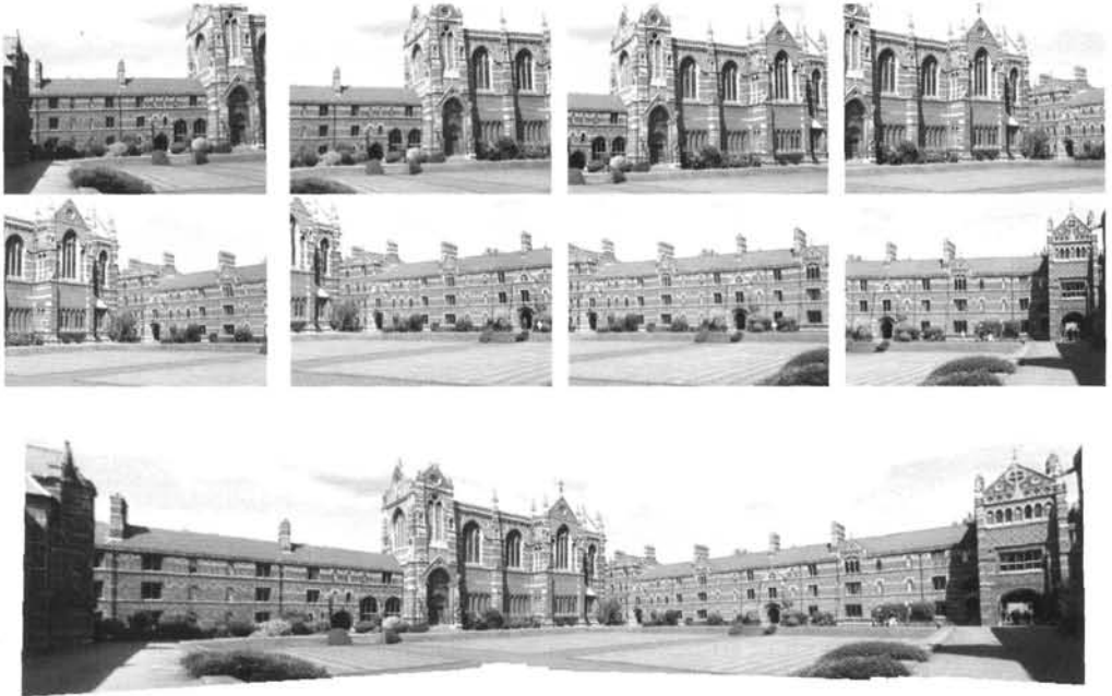
Fig. 8.9. Planar panoramic mosaicing. Eight images (out of thirty) acquired by rotating a camcorder about its centre. The thirty images are registered (automatically) using planar homographies and composed into the single panoramic mosaic shown. Note the characteristic “bow tie” shape resulting from registering to an image at the middle of the sequence.
