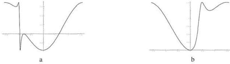
Fig. 12.4. (a) Example of a cost function with three minima. (b) This is the cost function for a perfect point match, which nevertheless has two minima.
