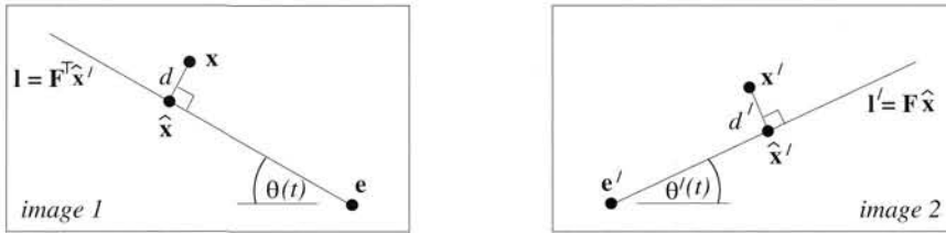
Fig. 12.3. The projections \hat{x} and \hat{x}' of an estimated 3D point \hat{X} lie on a pair of corresponding epipolar lines. The optimal \hat{x} and \hat{x}' will lie at the foot of the perpendiculars from the measured points x and x' . Parametrizing the corresponding epipolar lines as a one-parameter family, the optimal estimation of \hat{X} is reduced to a one-parameter search for corresponding epipolar lines so as to minimize the squared sum of perpendicular distances d^2 + d'^2 .
