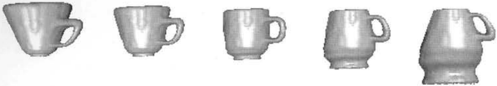
Fig. 1.4. Projective ambiguity: Reconstructions of a mug (shown with the true shape in the centre) under 3D projective transformations in the Z direction. Five examples of the cup with different degrees of projective distortion are shown. The shapes are quite different from the original.
