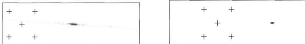
Fig. 5.6. Transfer of a point under the identity mapping for the normalized and unnormalized DLT algorithm. See also figure 4.4(p109) for further explanation.
