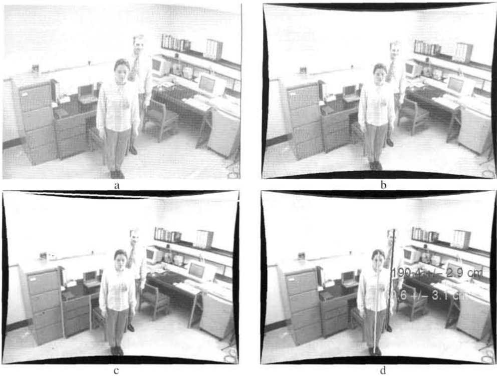
Fig. 8.21. Height measurements using affine properties. (a) The original image. We wish to measure the height of the two people. (b) The image after radial distortion correction (see section 7.4(p189)). (c) The vanishing line (shown) is computed from two vanishing points corresponding to horizontal directions. The lines used to compute the vertical vanishing points are also shown. The vertical vanishing point is not shown since it lies well below the image. (d) Using the known height of the filing cabinet on the left of the image, the absolute height of the two people are measured as described in algorithm 8.1. The measured heights are within 2cm of ground truth. The computation of the uncertainty is described in [Criminisi-00].
