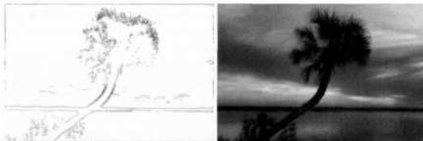
Figure 22.26. Scale selection mechanism: the left image shows the scale selected for each pixel of the image shown in Figure 22.25; the darker the pixel, the smaller the scale. A total of eight different scales were used to compute this image. The right image shows the local average computed for each pixel on the basis of the neighborhood selection mechanism.
