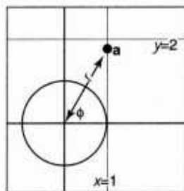
Figure 2.8. Polar coordinates for the point (x_a, y_a) = (1, \sqrt{3}) is (r_a, \phi_a) = (2, \pi/3) .
