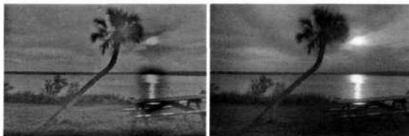
Figure 22.20. Images tonemapped by dividing by Gaussian blurred versions. The size of the filter kernel is 64 pixels for the left image and 512 pixels for the right image. For division-based algorithms, halo artifacts are minimized by choosing large filter kernels.
