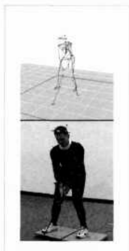
Figure 16.21. Optical motion capture: markers attached to a performer's body allow skeletal motion to be extracted. Image courtesy of Motion Analysis Corp.
