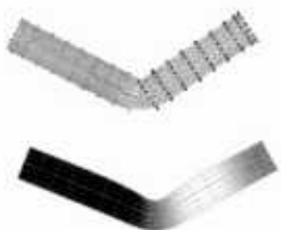
Figure 16.20. Top: Rigid skinning assigns skin vertices to a specific joint. Those belonging to the elbow joint are shown in black; Bottom: Soft skinning can blend the influence of several joints. Weights for the elbow joint are shown (lighter = greater weight). Note smoother skin deformation of the inner part of the skin near the joint.
