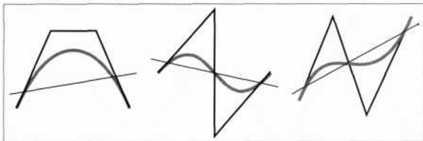
Figure 15.12. The variation diminishing property of Bézier curves means that the curve does not cross a line more than its control polygon does. Therefore, if the control polygon has no “wiggles,” the curve will not have them either. B-splines (Section 15.6.2) also have this property.
