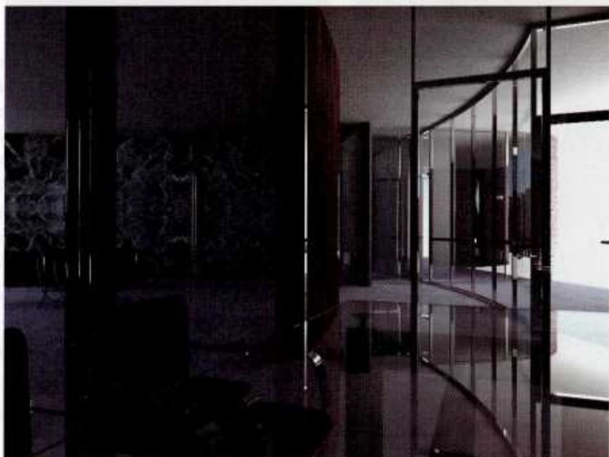
Plate XXV. Ray-traced and photon-mapped image of an interior. Most of the lighting is indirect. Image courtesy Henrik Jensen.
