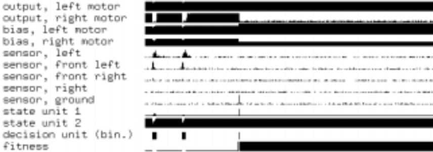
Figure 14. Activation values, motor biases, and fitness points during the 400 time steps of the evaluation trial for a robot controller of architecture E (experiment 1). The decision unit is illustrated as rounded to a binary value, with a black line corresponding to an active decision unit (activation exceeds 0.5, in which case the context network will be used) and white corresponding to an inactive decision unit (resulting in no use of feedback).
