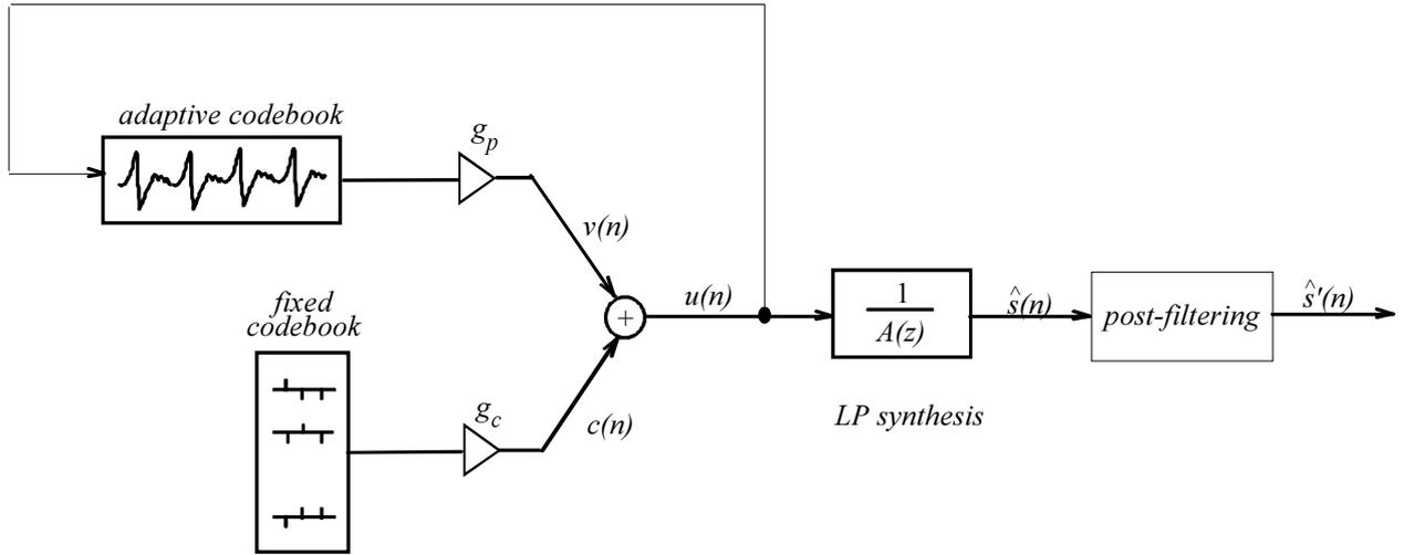
Figure 2: Simplified block diagram of the CELP synthesis model
