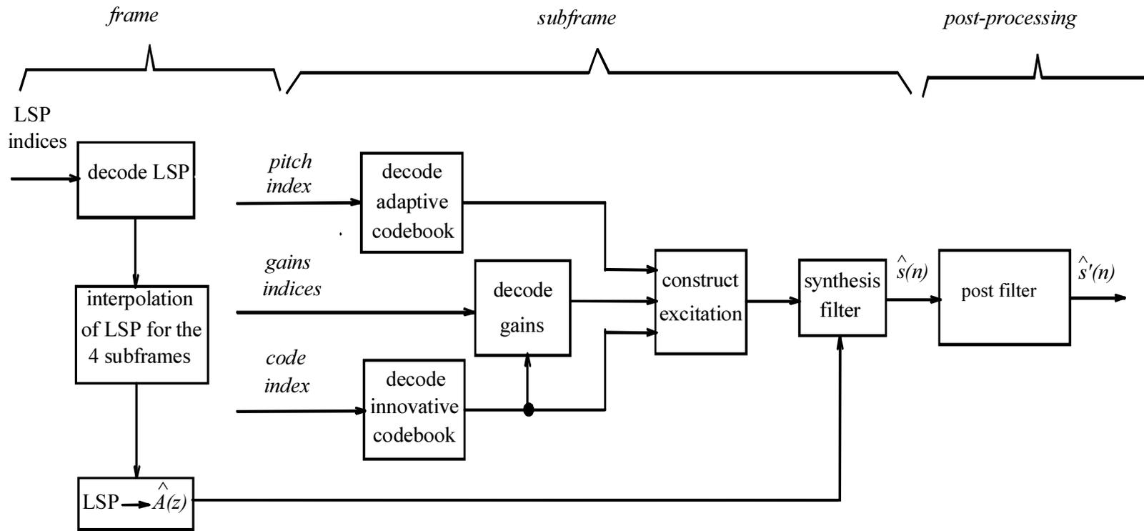
Figure 4: Simplified block diagram of the GSM enhanced full rate decoder
